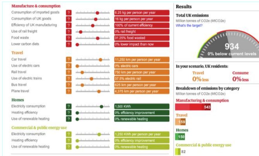
FIGURE 6: AN EXAMPLE OF “SLIDERS” (ON THE LEFT), WHICH ALLOW INPUT VALUES TO BE CHANGED, USED TO INVESTIGATE THE BEHAVIOUR OF SYSTEM OUTPUTS (ON THE RIGHT)
